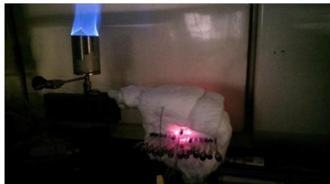
Figure 5: A Swiss-roll reforming propane with a blue flame and a bright center reaction zone.
