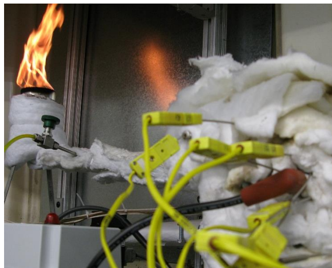
Figure 7: Side view of Swiss-roll reformer with flare visible.
