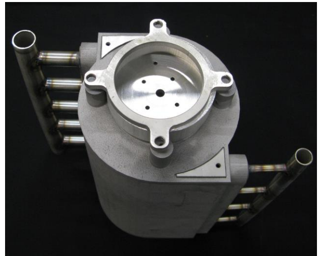
Figure 2: The Swiss-roll fuel reformer prototype, manufactured by an additive manufacturing technique known as Direct Metal Laser Sintering (DMLS), integrated with accessory components.
